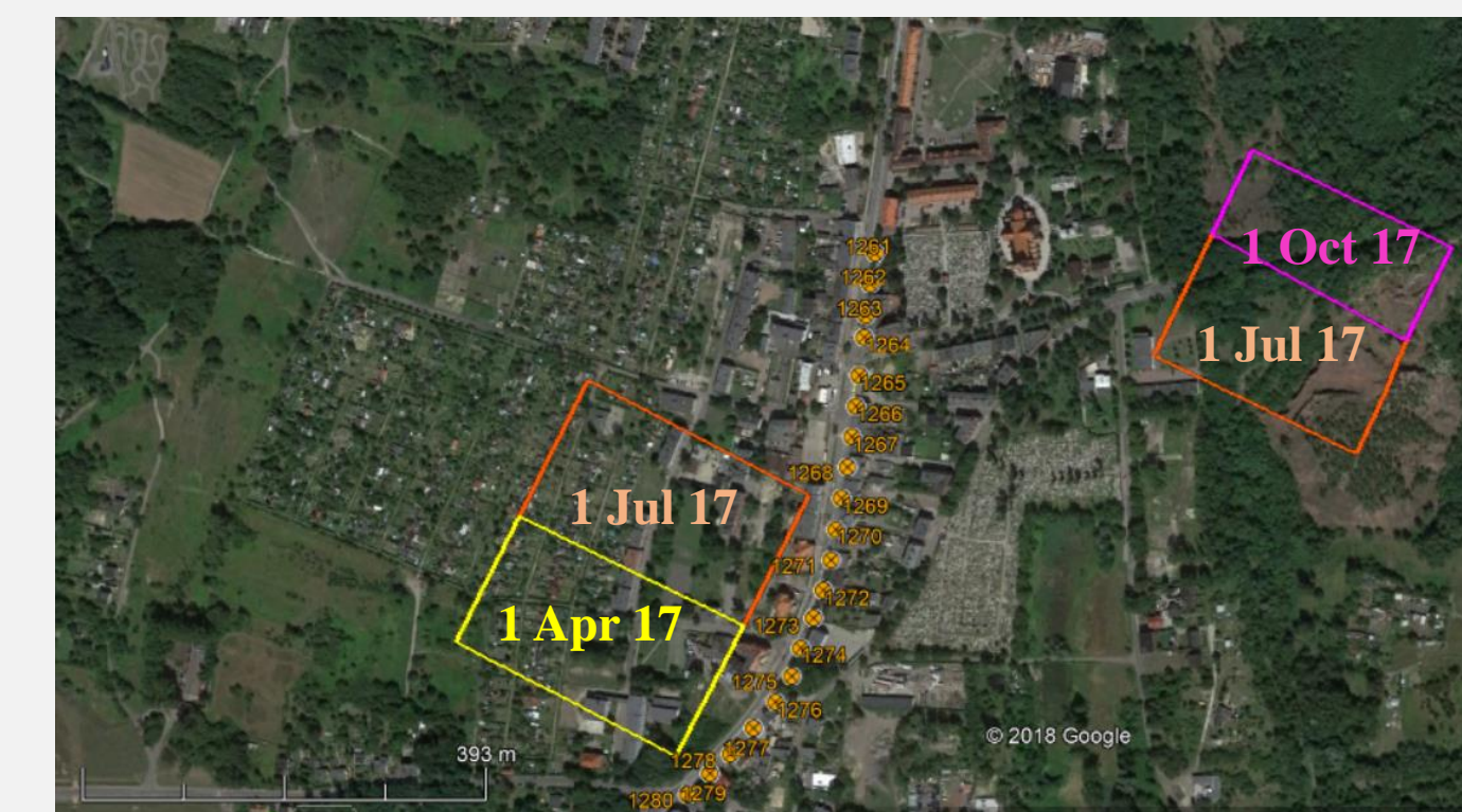
Fig. 2. View of Wirek-II area with levelling benchmarks and polygons of coal extraction
