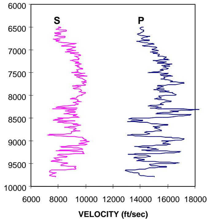
Figure 3. Velocity logs of Cotton Valley section.
