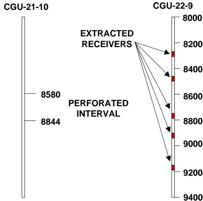
Figure 1. Receiver configuration for extracted 5-level system for upper Cotton Valley test.
