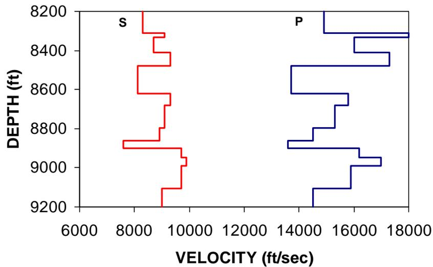
Figure 4. Layered velocity structure for advanced analyses.
