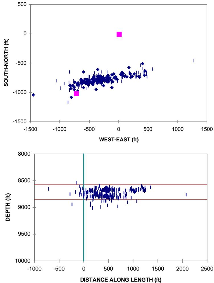
Figure 2. Plan view and side view maps of Stage 3 (upper) Cotton Valley fracture test.
