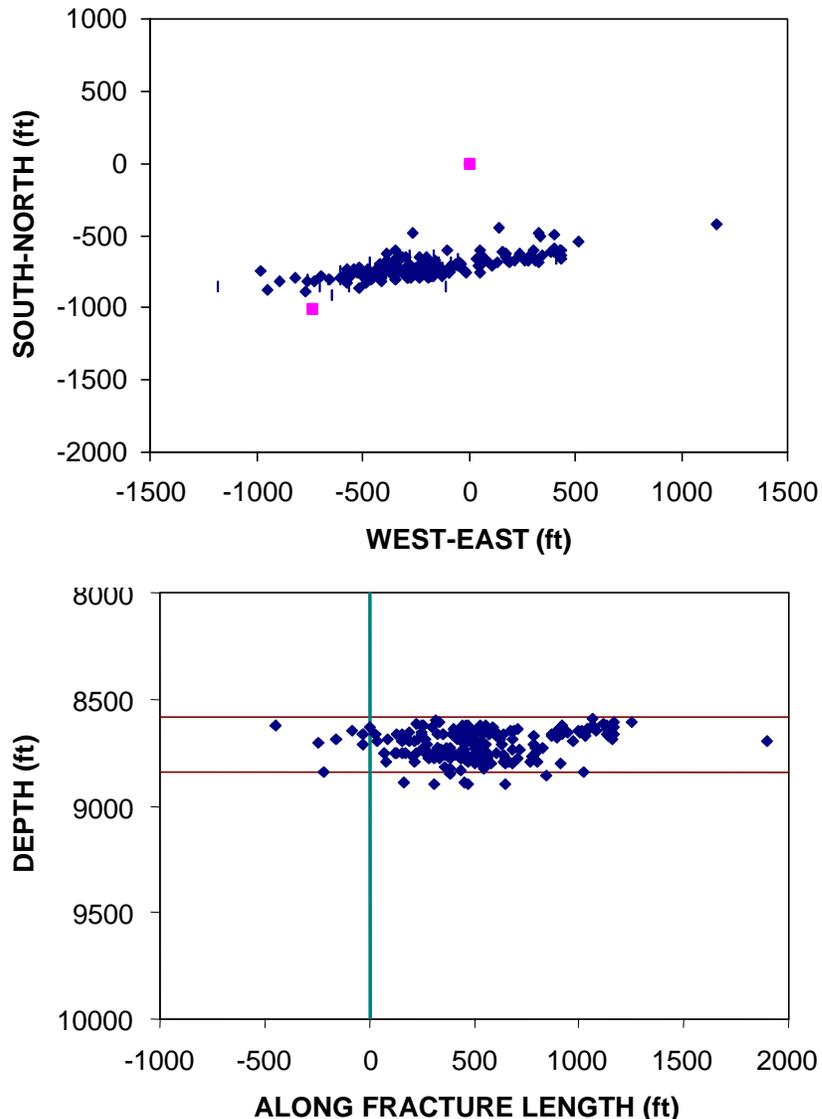
Figure 5. Plan view and side view maps of upper Cotton Valley stimulation using velocity structure.
