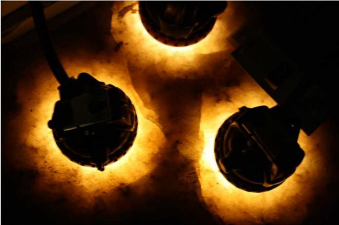
Figure17: Observation of the "glazing" effect of the surface by light transmission.
