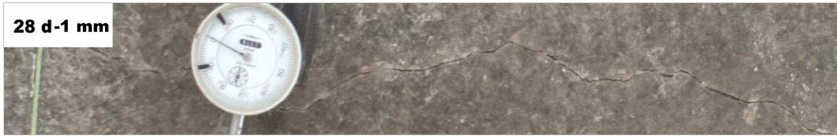
**Figure19:** Measurement of the main crack opening at the end of the 3<sup>rd</sup> cooling cycle using a comparator. The opening is measured at 1 mm after 28 days' cooling.
