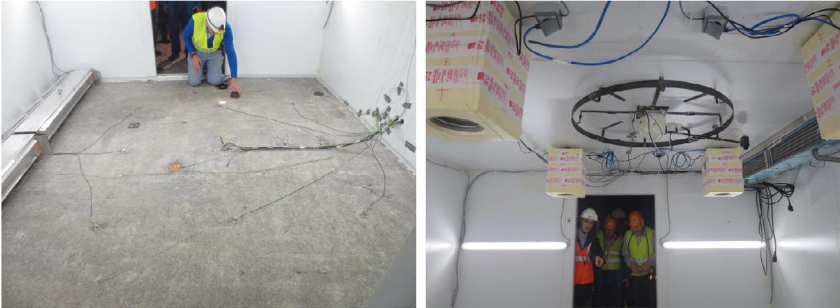
**Figure5:** Left: Picture of the temperature sensors, strain gauges, heat flow sensor and ultrasound sensors on the room surface. To the right, on the room ceiling, the 4 heat-protected digital cameras, thermal camera on its carousel and LED lighting at different places on the door.
