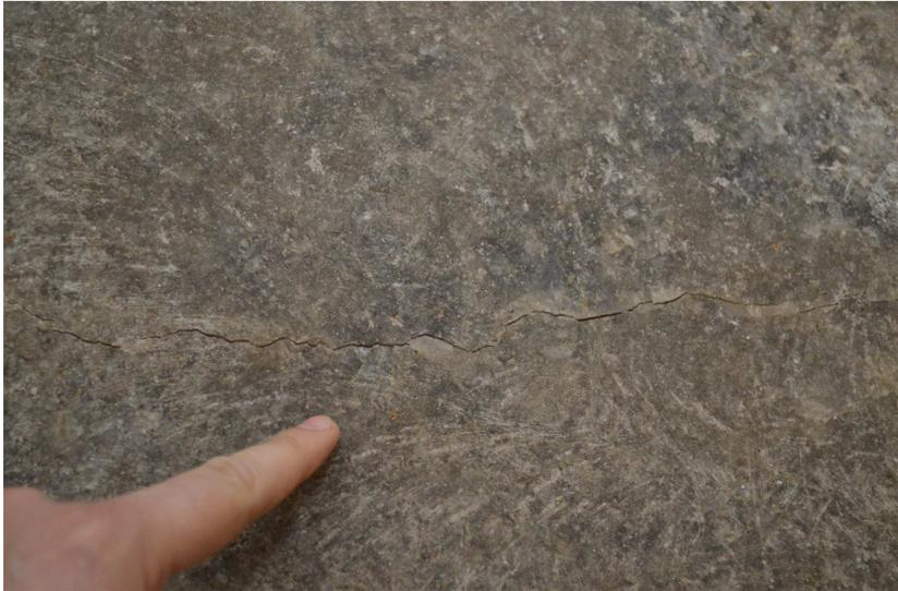
**Figure15:** the first crack a few hours after cooling had started
