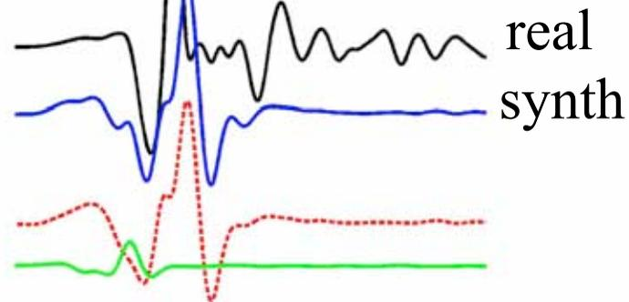
The stopping phase (red) exerts the primary control on the waveform
