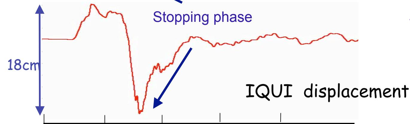
Accelerogram filtered from 0.01 to 1 Hz and integrated
