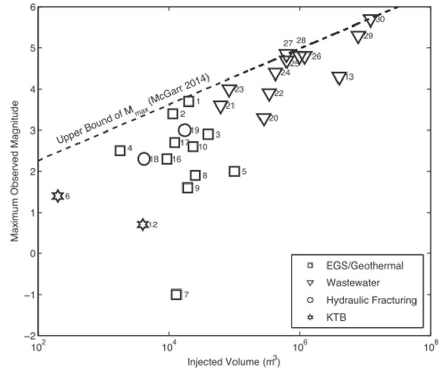
**Fig. 1.** Observed maximum magnitude of seismic events in geothermal operations (squares), wastewater disposal wells (triangles), hydraulic fracturing (circles), and fluid injection in the KTB scientific well (stars) as functions of volume of injected fluid. Numbers by symbols correspond to the order in which data are listed in [Table 2](#).
