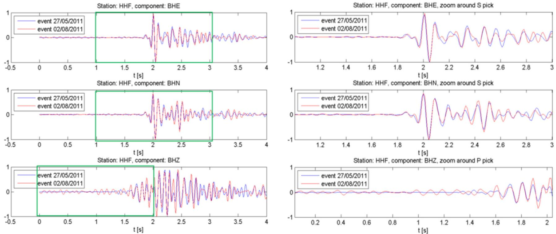
Figure 13. Filtered waveforms of the May 27, 2011 and August 2, 2011 events at station HHF. The green rectangles in the left plots are enlarged in the right plots. Waveforms start 2 seconds before the S-wave pick. The waveforms are aligned on the S-wave pick. Each trace is normalized to its maximum.
