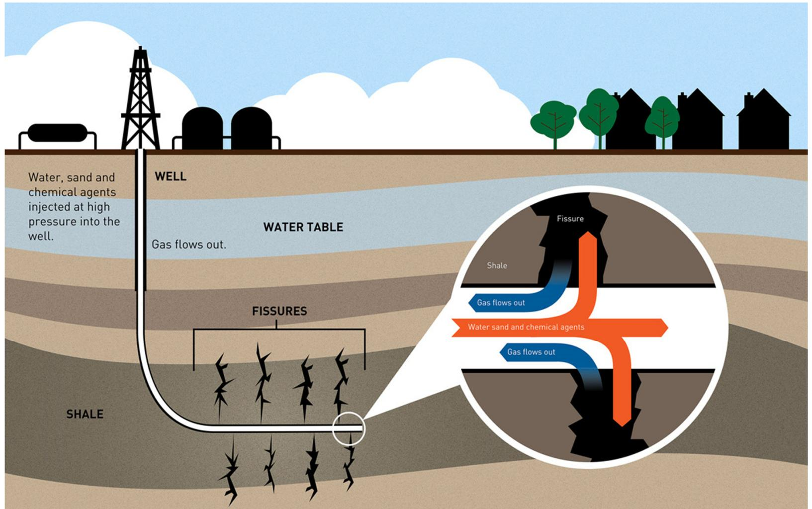
Schematic diagram showing the general features of a fracking operation; <http://publisher.attn.com/>
