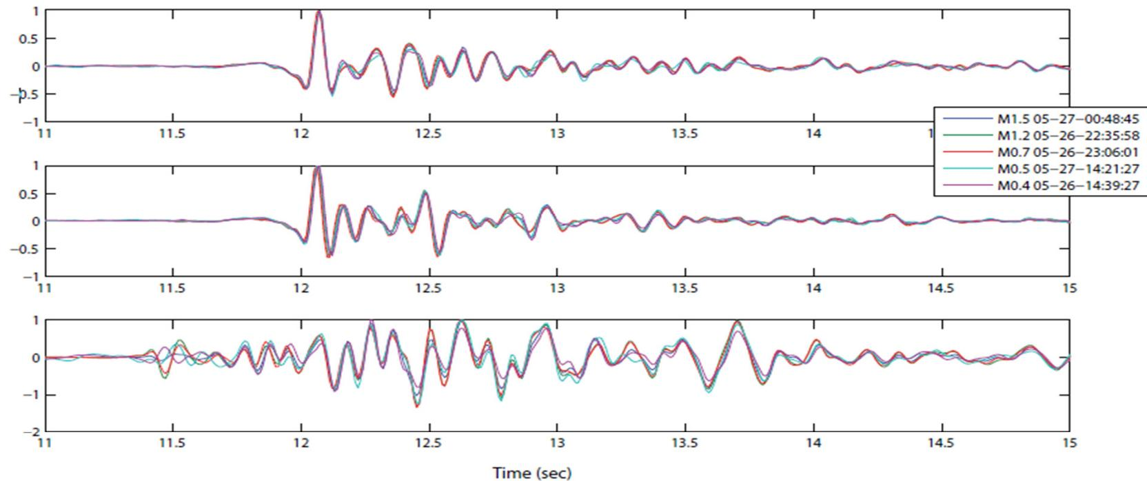
**Figure 28: Traces of seismic events vs time, observed on the local station HHF, normalized on maximum amplitude. The two upper diagrams show the horizontal components, which picked up the shear waves and the lower diagram shows the vertical component with the compressional wave. The records are remarkably similar in shape, showing that all events originated from the same source plane.**
