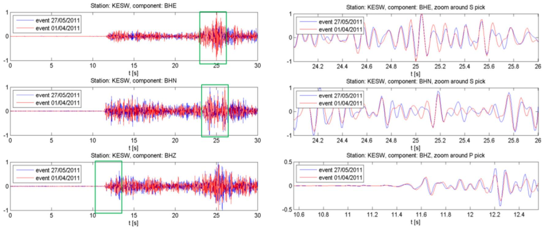
Figure 9. Filtered waveforms of the April 1, 2011 and May 27, 2011 events at station KESW. The green rectangles in the left plots are enlarged in the right plots. Waveforms start 25 seconds before the approximate S-pick. The waveforms are aligned on the S-pick and the difference on the P-pick is about 0.02 s. Each trace is normalized to its maximum.
