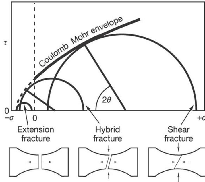
Diagram showing that for high differential stress (bigger stress circle, right), the rock will fail in shear, whereas for low differential stress (small circle, left) the failure mode will be tensile; <http://www.nature.com/>
