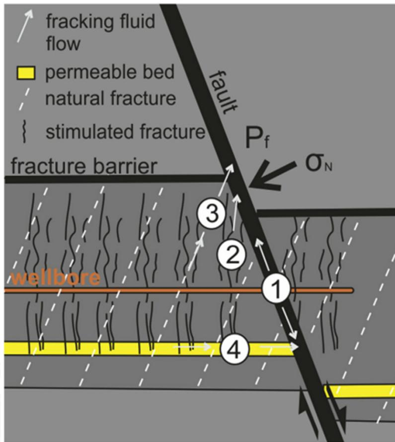
Potential mechanisms for the transmission of a pore fluid pressure pulse or fluid into a fault to cause reactivation:
