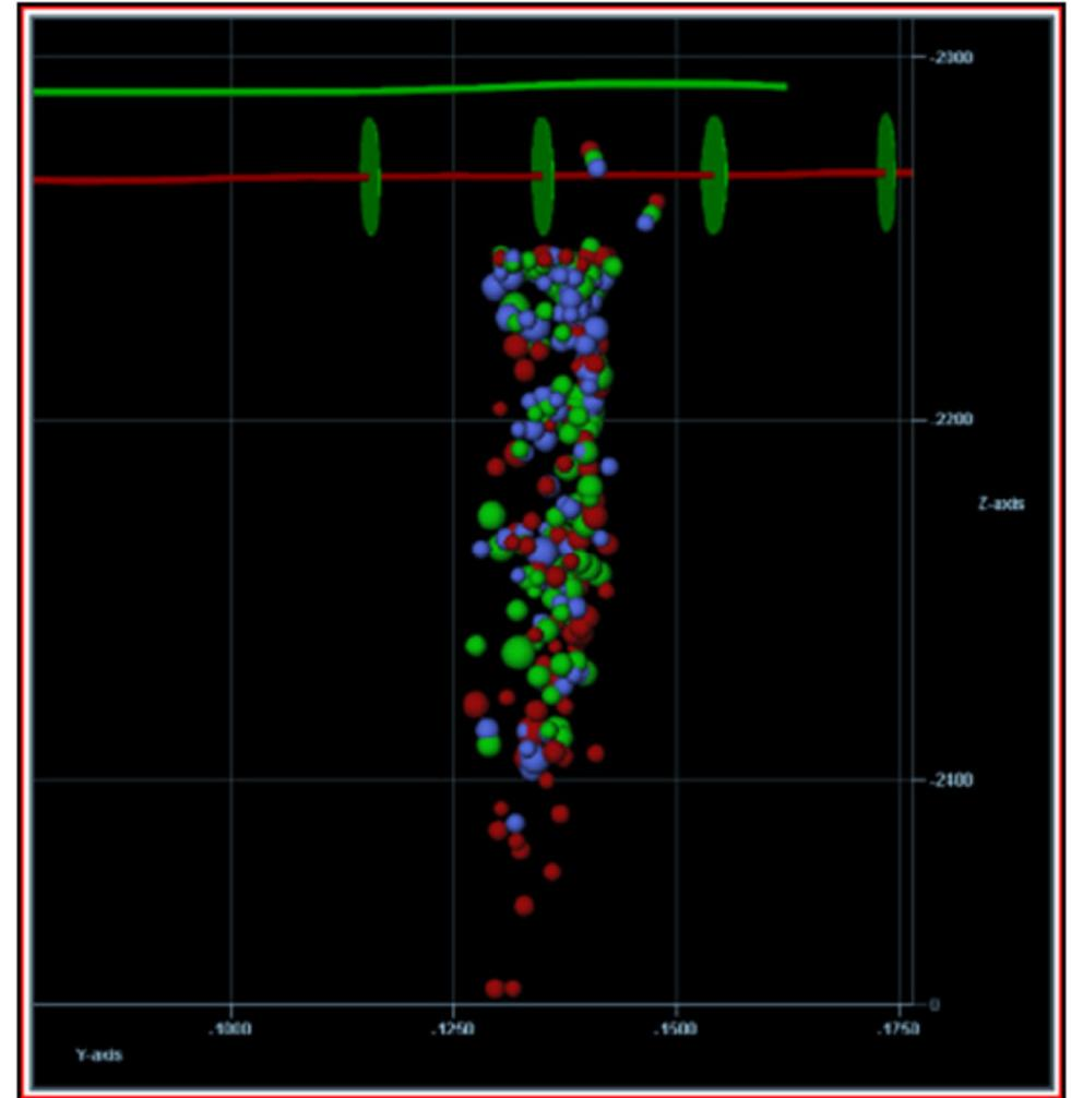
Micro-seismicity events (coloured circles) and hydraulic fracture stages (green ellipses) along horizontal wellbore legs ; Oil and Gas Commission open report, August 2012
