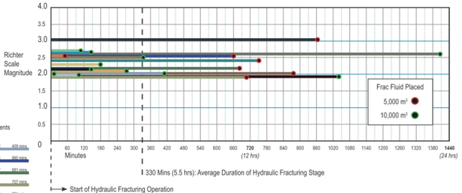
Timing of seismicity events, resulting from fluid injection at selected hydraulic fracturing stages. Green dots designate events linked to stages with 10,000 m<sup>3</sup> total 'Fracturing Fluid Placed' (two injections of 5000m<sup>3</sup> separated by one hour). Red dots are events linked to stages with 5,000 m<sup>3</sup> total 'Fracturing Fluid Placed'; Oil and Gas Commission open report, August 2012
