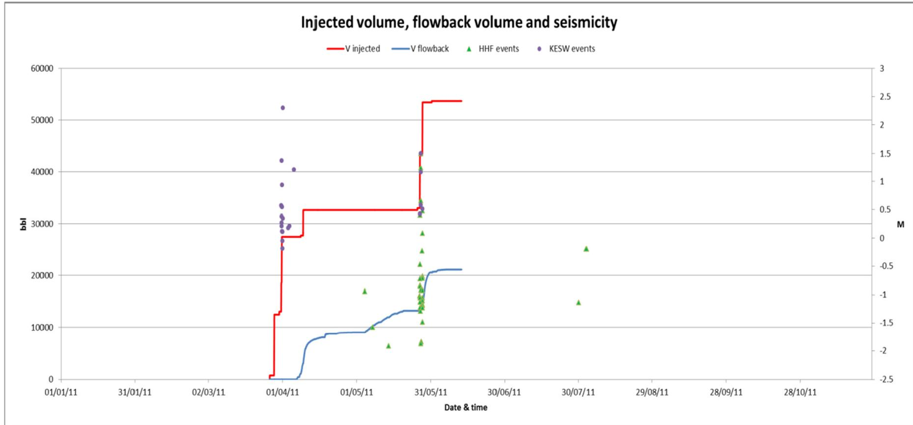
Figure 20. Injected volume and flowback volume in the exploration well Preese Hall. Events detected by KESW and by HHF.
