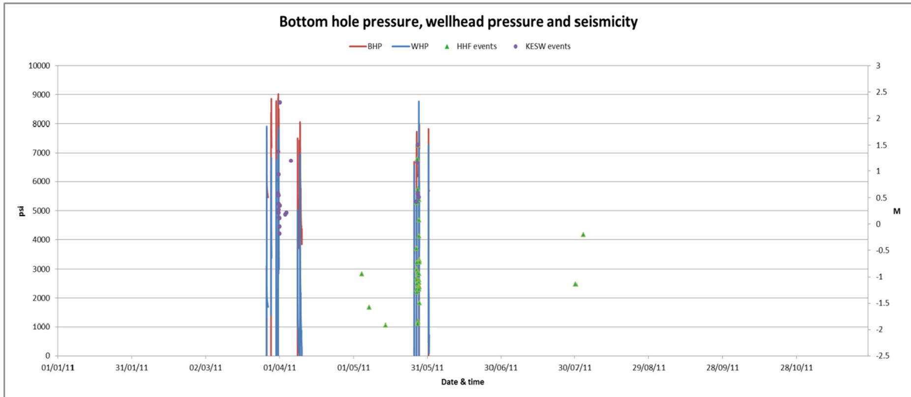
Figure 18. Bottom hole pressure (BHP) and wellhead pressure (WHP) in the exploration well Preese Hall. Events detected by KESW and by HHF are represented by the origin time and magnitude relative to the May 27, 2011 master event. The station HHF was operating since April 12, 2011 but is able to record much smaller events.
