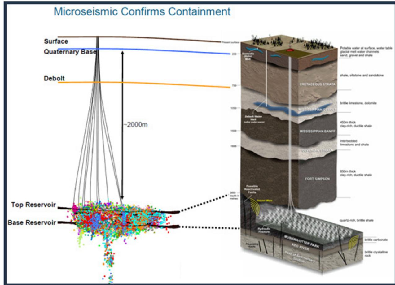
Cumulative microseismic plot for Kiwigana, coloured dots indicate contained micro-seismicity events caused by tensile and shear failure of intact shale. Trail of coloured dots suggest reopening or movement of pre-existing fault. Generalized stratigraphic column to right, NRCan; Oil and Gas Commission open report, August 2012
