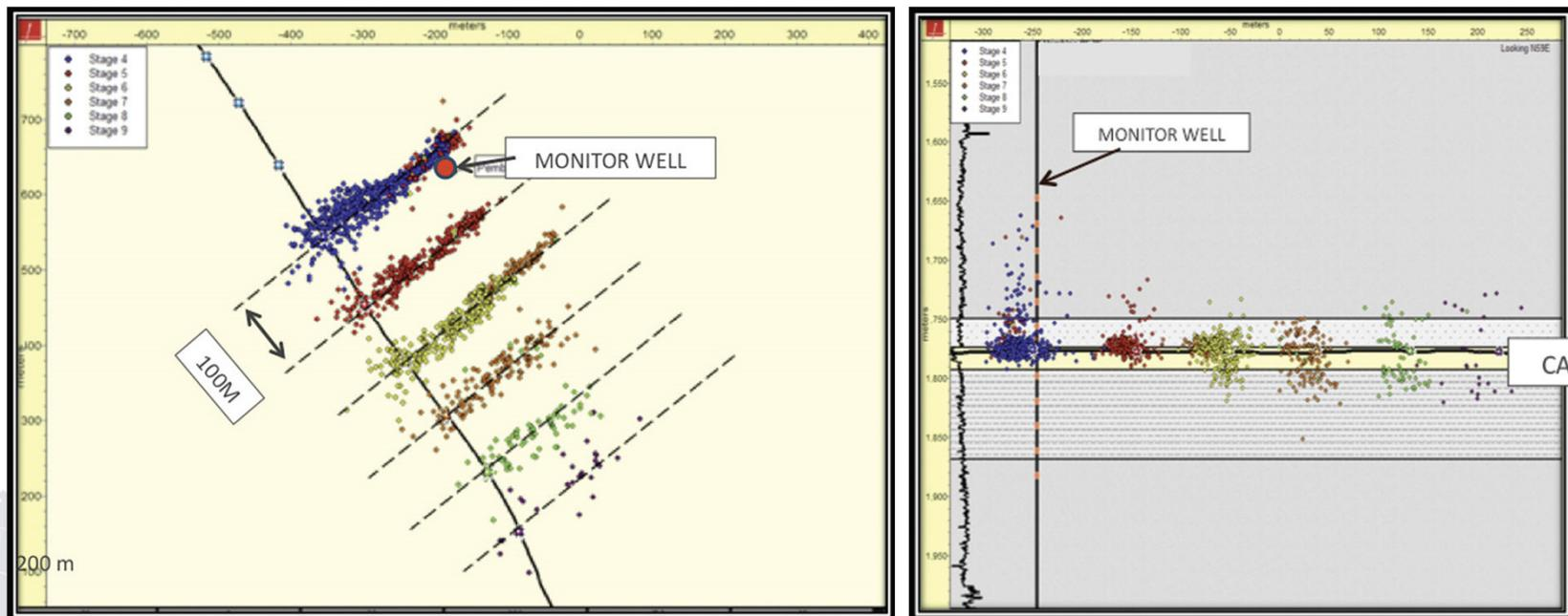
Map view (left) and cross section (right) of fracking stages and seismicity from West Central Alberta, Canada
