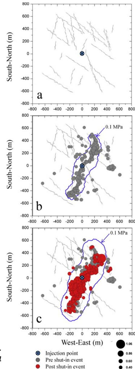
Discrete fracture network model with pore fluid flow algorithm.
