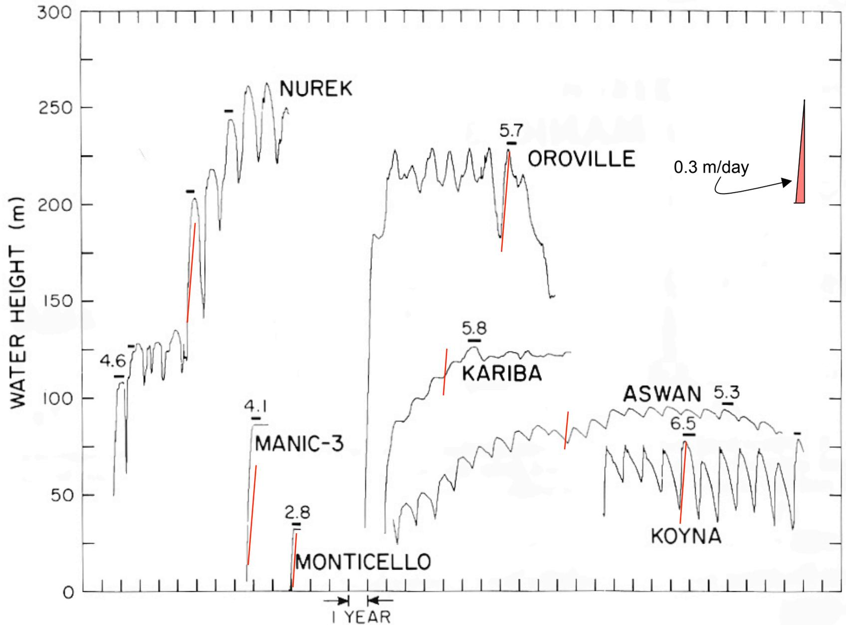
Simpson, Leith and Scholz, 1988 - Two types of Reservoir Induced Seismicity
