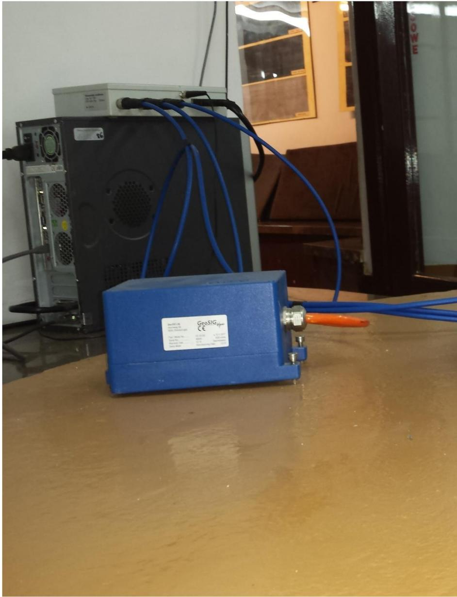
**Calibration of a vibrations' registration apparatus used within the GRSS seismic network**
